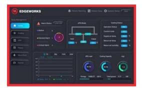
Edge Monitoring solution adopts the all in one monitoring host with built in communication ports, display panel, and management software.
